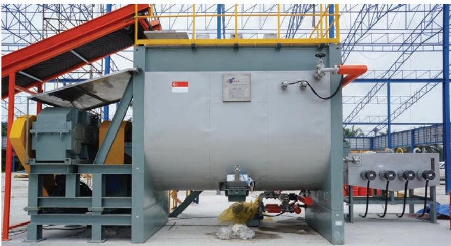
The digester, which works at 80°C to break down organic waste into fertilizer, is an integral part of Biomax’s process.
